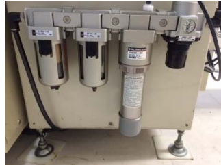
Excess dryer units connected to air circulation system were removed for energy saving (E&D center)
